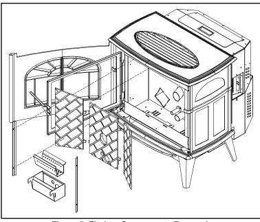
Figure 5: Firebox Components Removal.
