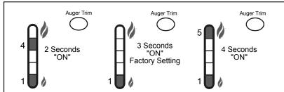
Figure 3: Auger trim and heat level indicator.
