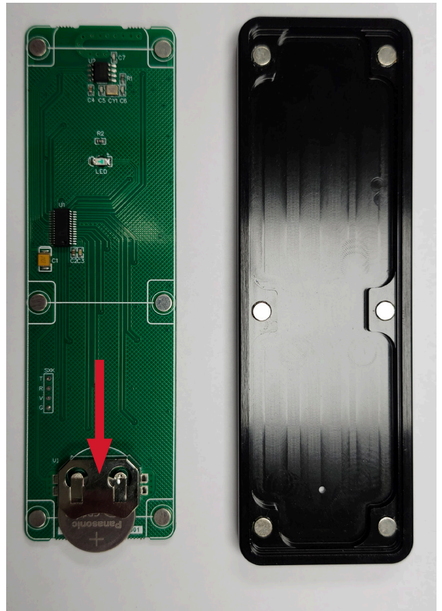
Figure 41: Remote Battery - Step 3
