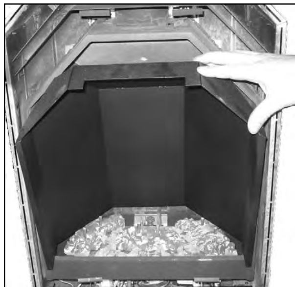
Figure 53. Bottom of Steel Line Put in Place.
