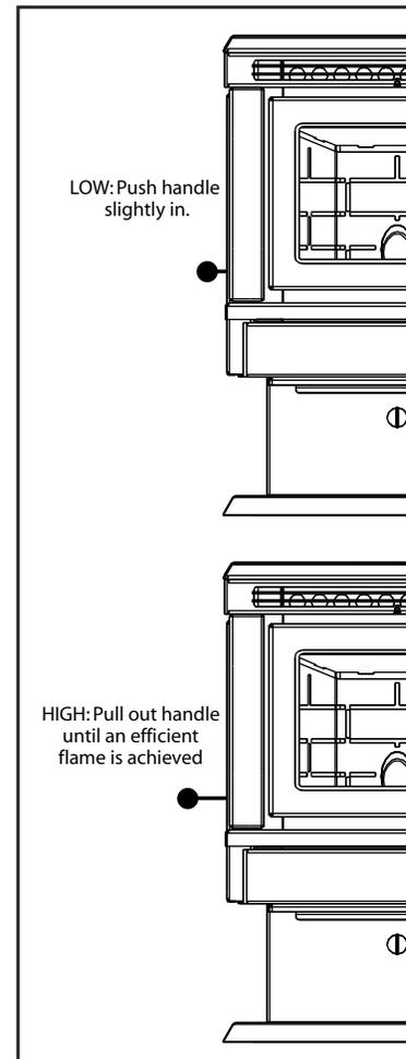
Figure 1: Slider / damper positions.
