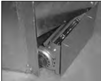
Figure 48: Installing Fan Through the Back.
