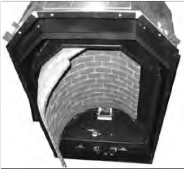
Figure 54. Slid In the Ceramic Liner.
