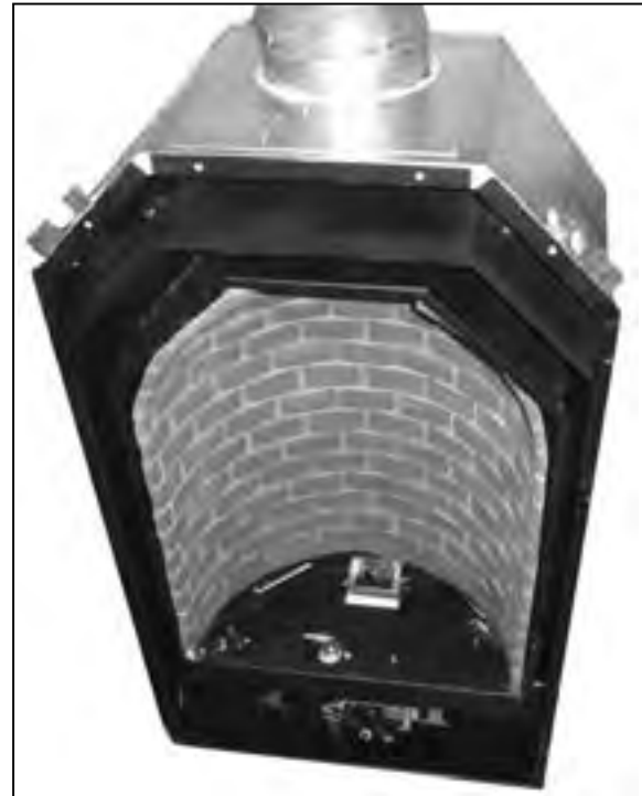
Figure 55. Ceramic Line Put in Place.
