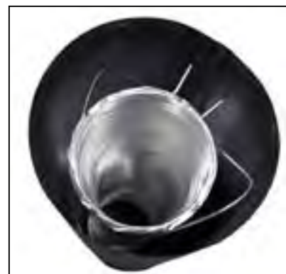
Figure 27: Wire Spacer in Place.
