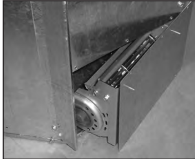
Figure 46: Installing Fan Through the Back.
