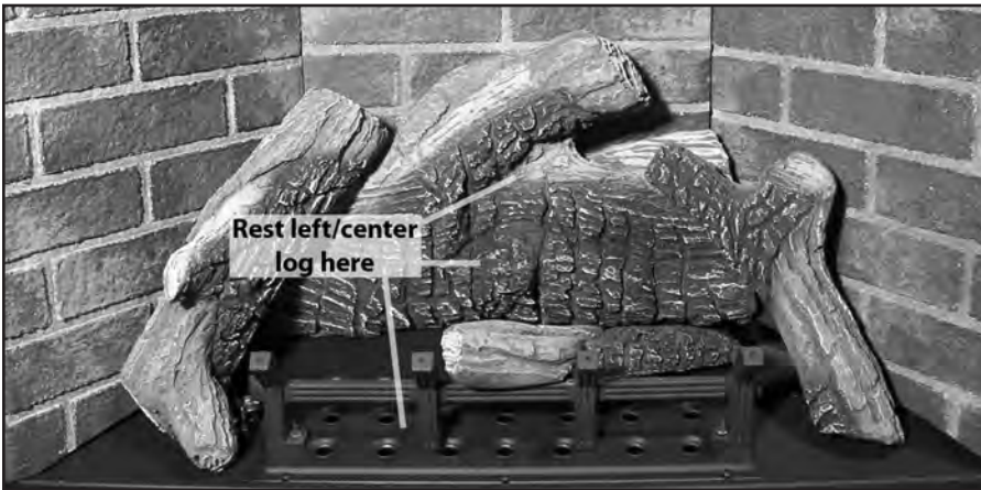
Figure 45. Fourth Stage Log Set Installation.
