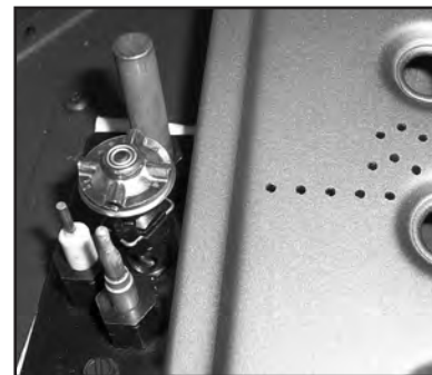
Figure 15: Burner to pilot hood relationship.
