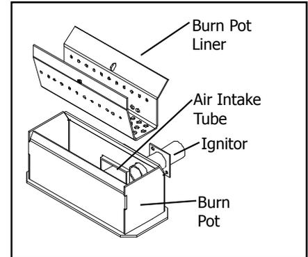
Figure 8: EF5 Burn pot and Liner
