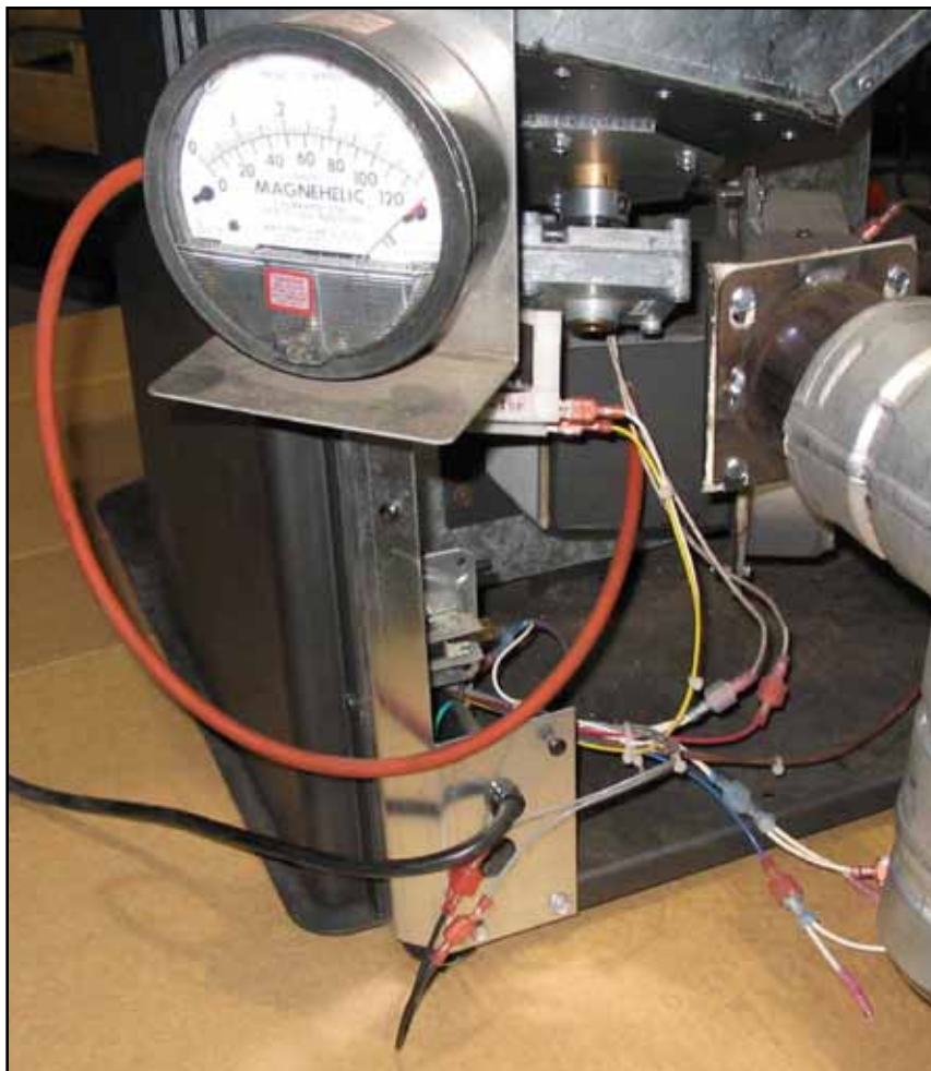
Figure 39: Measuring The Vacuum Level Produced By The Exhaust Blower.
