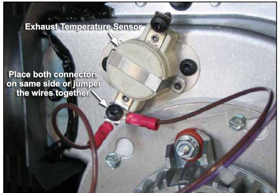
Figure 31: By-Passing The Exhaust Temperature Sensor/ Switch (EF 3 Shown).
