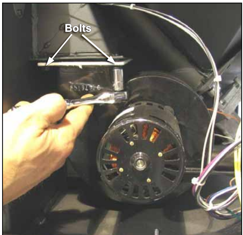
Figure 27: Removing The Convection Blower.
