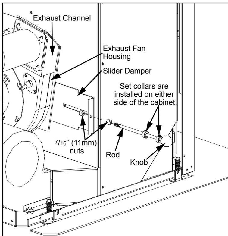
Figure 20: Slider/Damper Plate & Rod in Unit.
