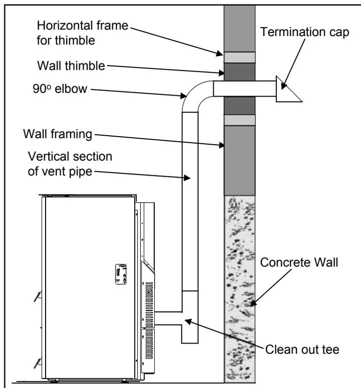
Figure 15: Venting with concrete wall behind unit .
