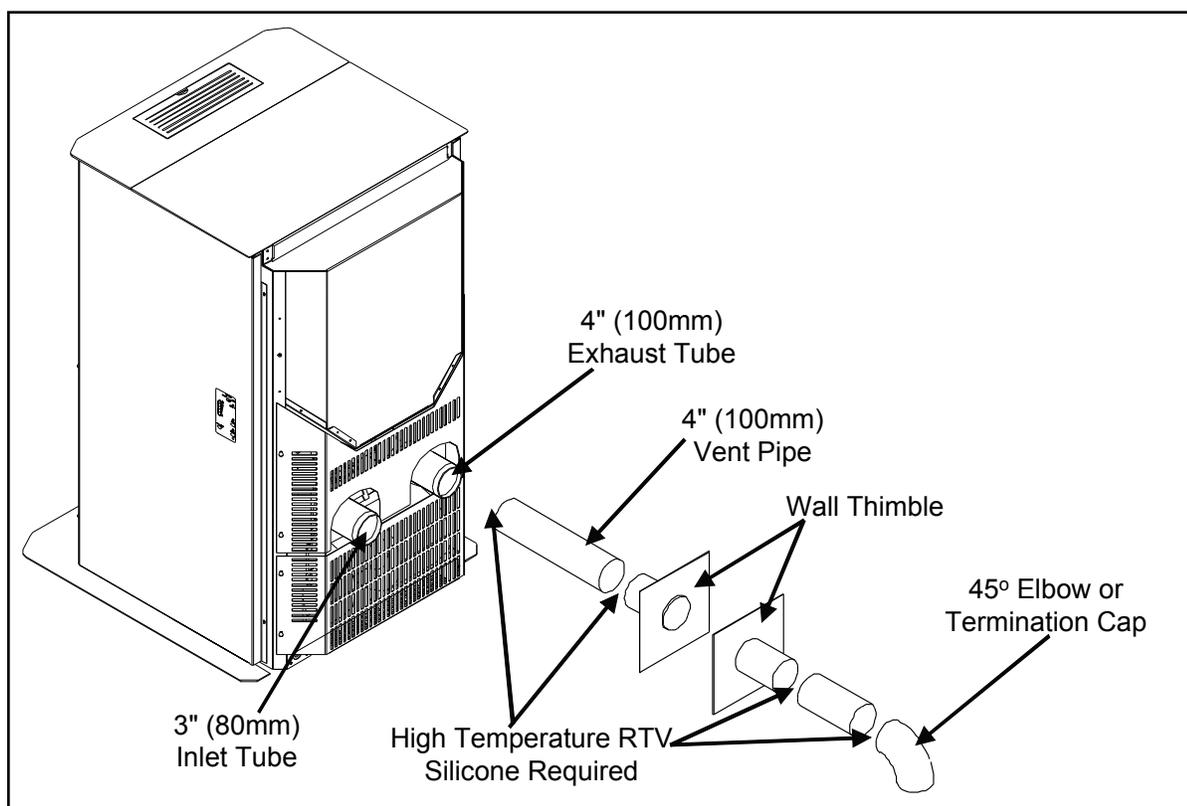
Figure 12: Straight through wall Installation.
