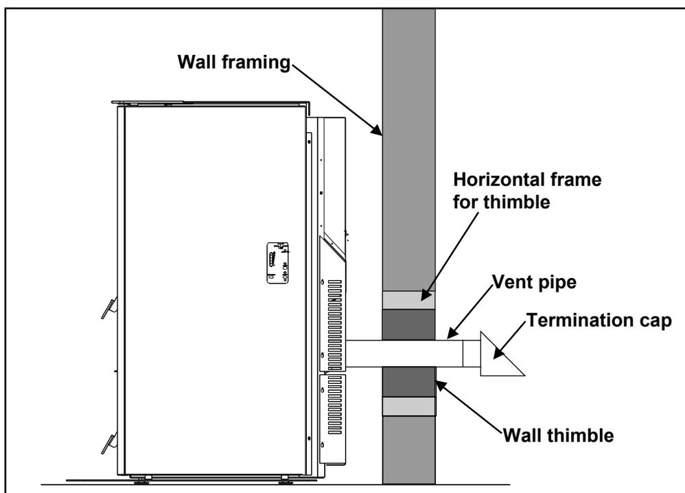
Figure 13: Straight through Wall Installation - Side View.
