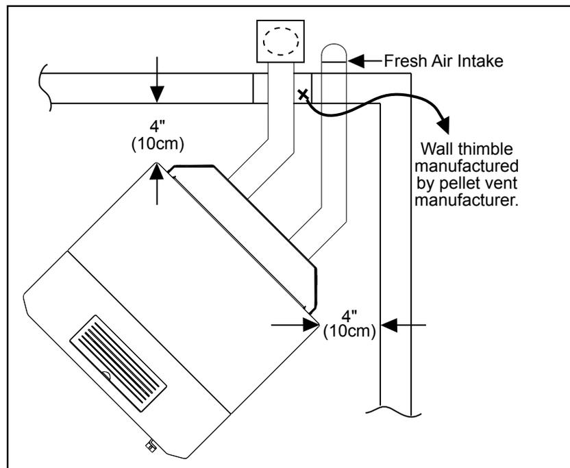
Figure 11: Corner Installation.
