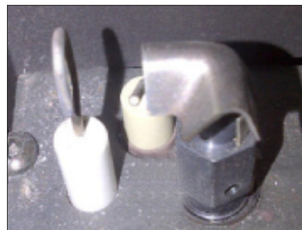
Figure 20: Proper Pilot Position
