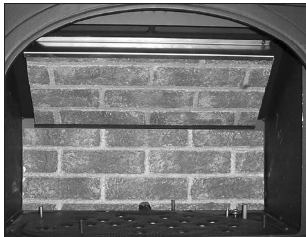
Figure 64: Back brick panel in place.
