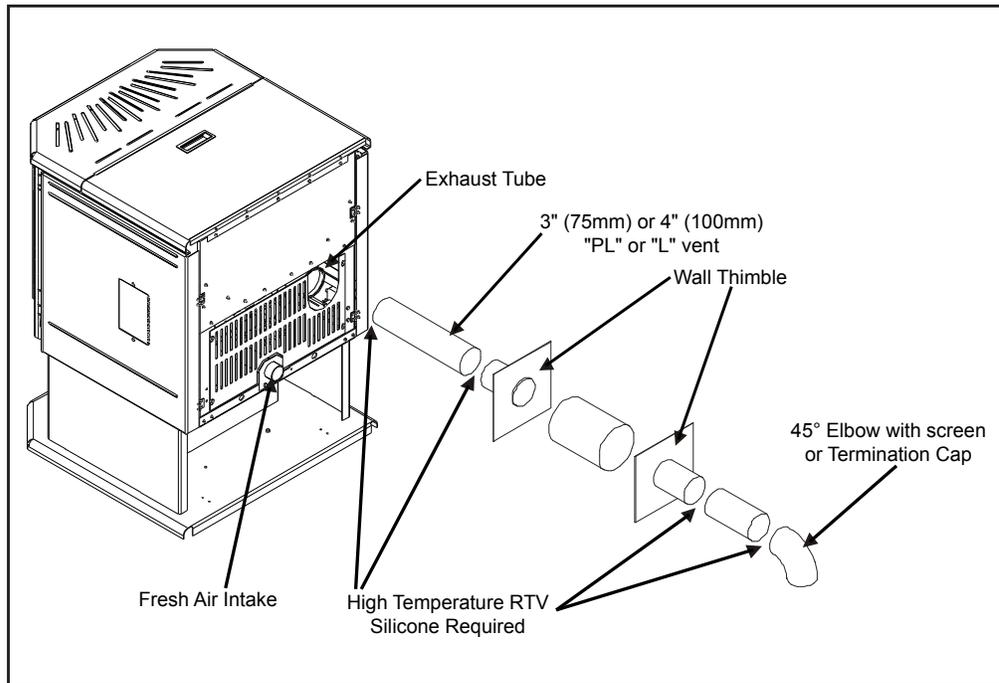
**Figure 28: Straight through wall Installation.**
