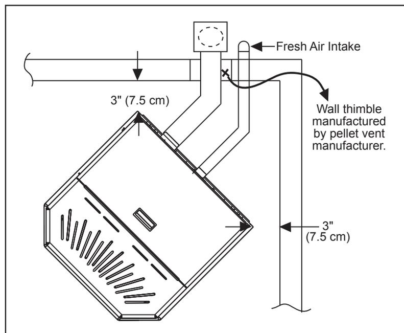
Figure 27: Corner Installation.
