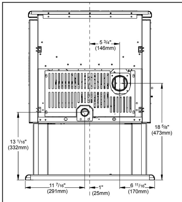
**Figure 24: Meridian Freestanding Inlet and Outlet Location.**
