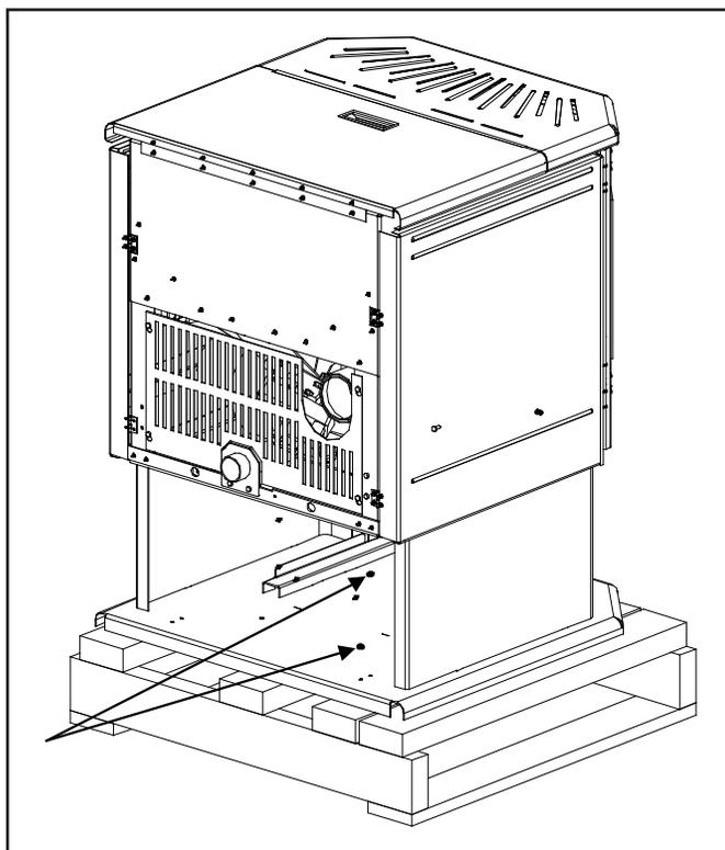
Figure 11: Removing Freestanding Stove From the Pallet.
