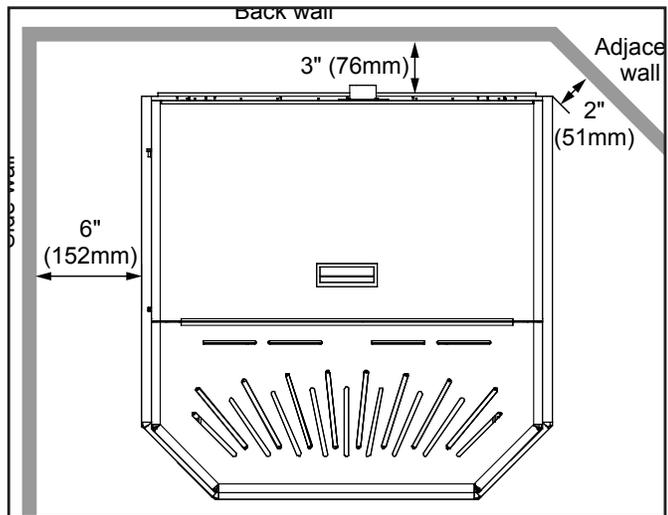
**Figure 16: Minimum Clearances to Combustibles for Freestanding Meridian.**
