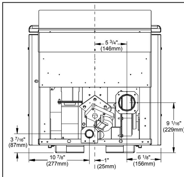
**Figure 25: Meridian Insert Inlet and Outlet Location.**
