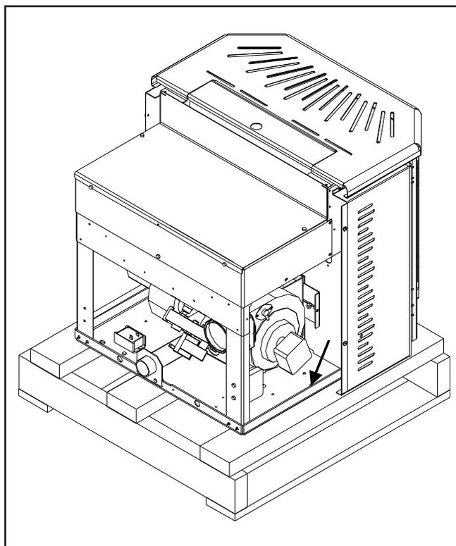
Figure 12: Removing Insert Stove From the Pallet.
