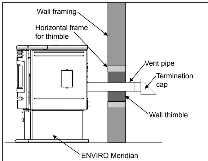
**Figure 29: Straight through Wall Installation - Side View.**
