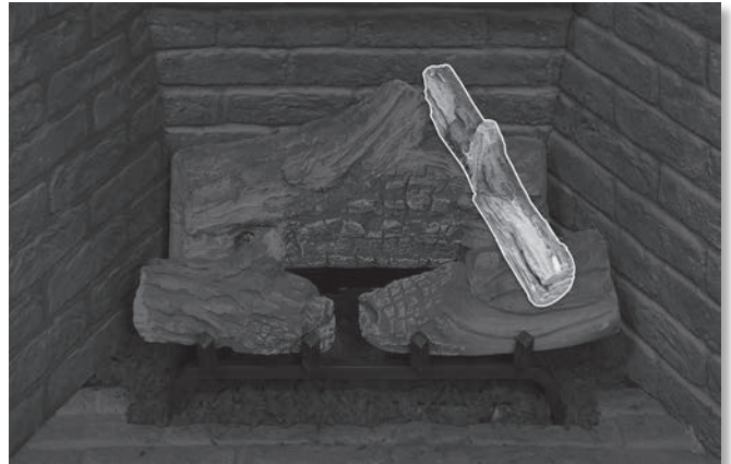
Figure 80: Log Set Installation - Step 4
