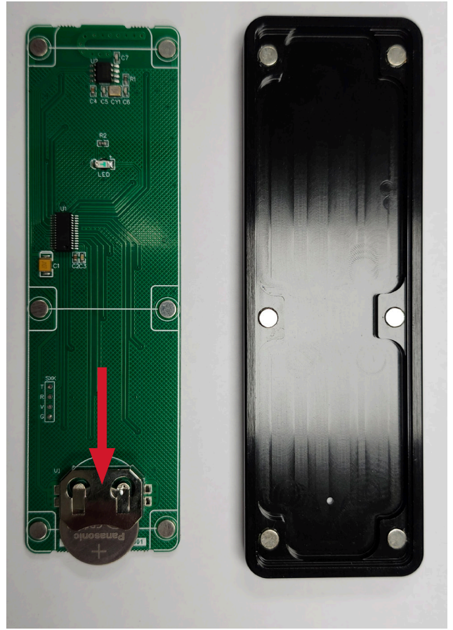
Figure 32: Remote Battery - Step 3
